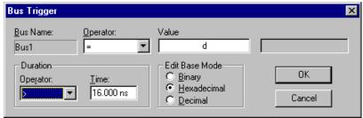
With the "<" operator, the minimum time is either twice the sample period or the absolute minimum of 16 ns. With the ">" operator, the minimum time is either equal to the sample period or the absolute minimum of 8 ns. The entered time will be rounded to a multiple of the sample period.
